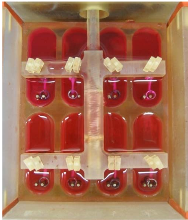
Figure 4-2: View of tissue chamber within stretch bioreactor depicting eight tissue samples coupled to H-shaped arm. Each tissue well is filled with tissue culture medium. Details on how the tissue samples are attached are compiled in Section 4.3.1 .
